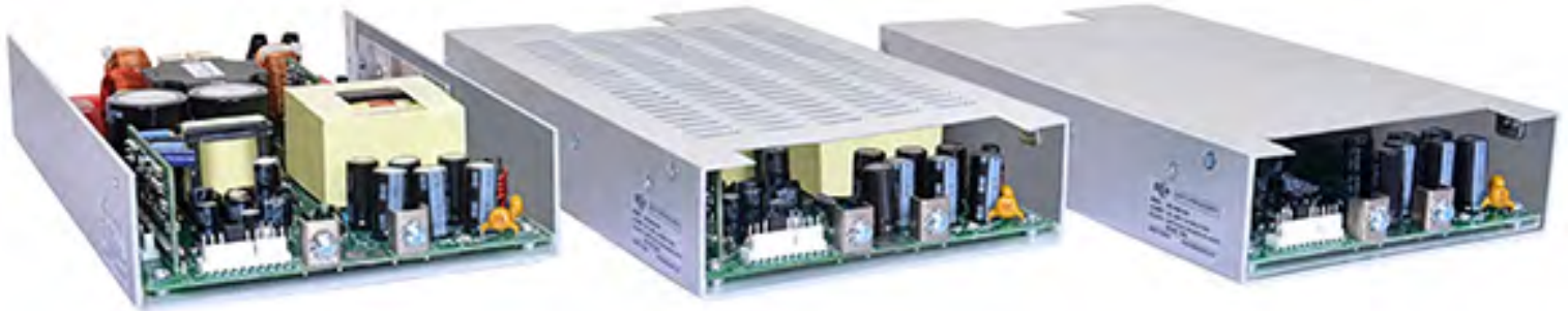
Figure 5: The VSP600 series is available in three package configurations with different nominal power ratings; 600-watt convection cooled U channel units, 420-watt slotted cover units, and 360 watt plain cover units. (Image source: Bel Power Solutions)
