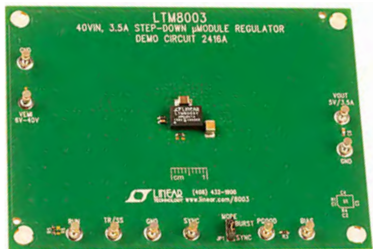
Figure 10: The DC2416A demo board simplifies connection with and evaluation of the LTM8003 Silent Switcher device. (Image source: Analog Devices)
