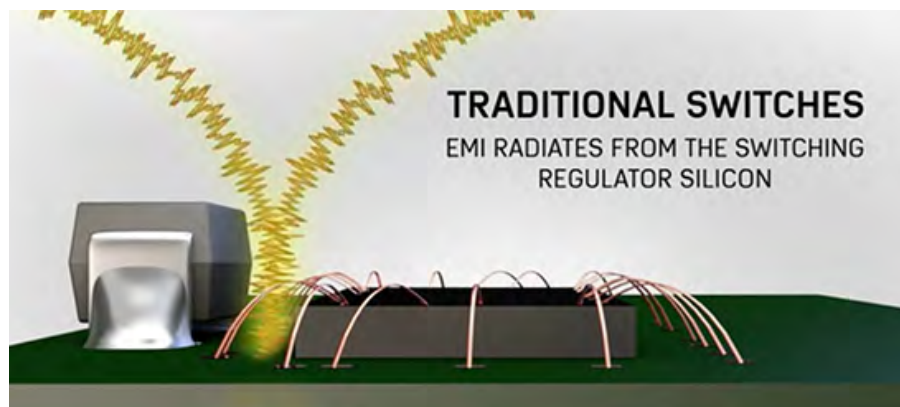
Figure 3: The bond wires from the IC die to the package function as miniature antennas and radiate undesired RF energy. (Image source: Analog Devices)
