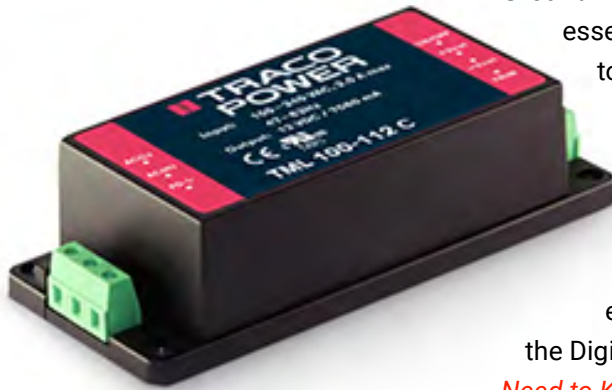
Figure 3: Shown here is a TML 100C Series, 85-100 Watt AC-to-DC power module from Traco Power. Active power-factor correction (PFC) ensures a power factor of better than 0.95 (for 230 VAC) and better than 0.99 (for 115 VAC). (Image source: Traco Power)
